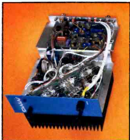
A 600W solid-state VHF module.
