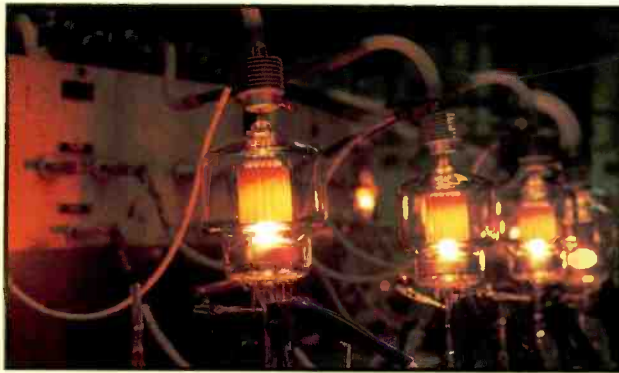
A critical part of power tube construction involves the bake-out procedure, in which residual gas is burned out of the assembly.
