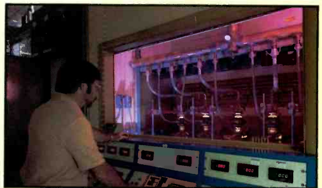
Testing of power-grid tubes involves both dc and RF measurements. Through careful design and construction, production variations in operating parameters can be minimized.
