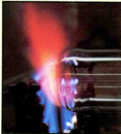
The production of power vacuum tubes is perhaps as much art as science. Shown is one of the glass-blowing stages used in making the envelope for a medium-power tube.
